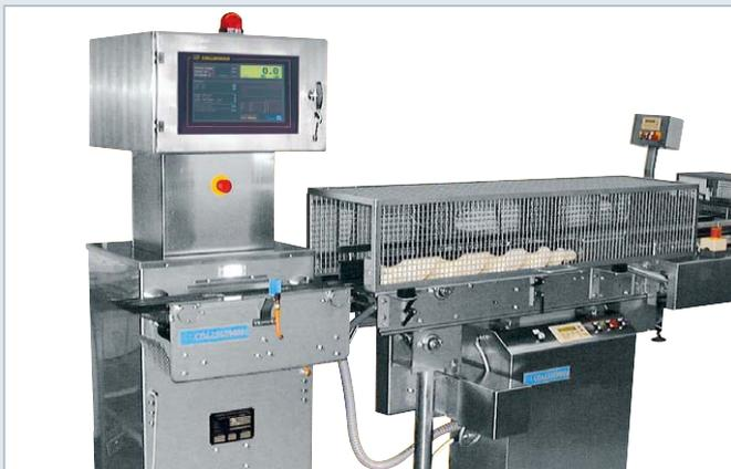
For the use in extremely rough environmental conditions (e.g. wet rooms) we offer the water jet proof checkweigher **TC 8500**. In the tinned food industry this type has produced an output of up to 450 weighings per minute for many years. The whole machine is washable with high water pressure.
