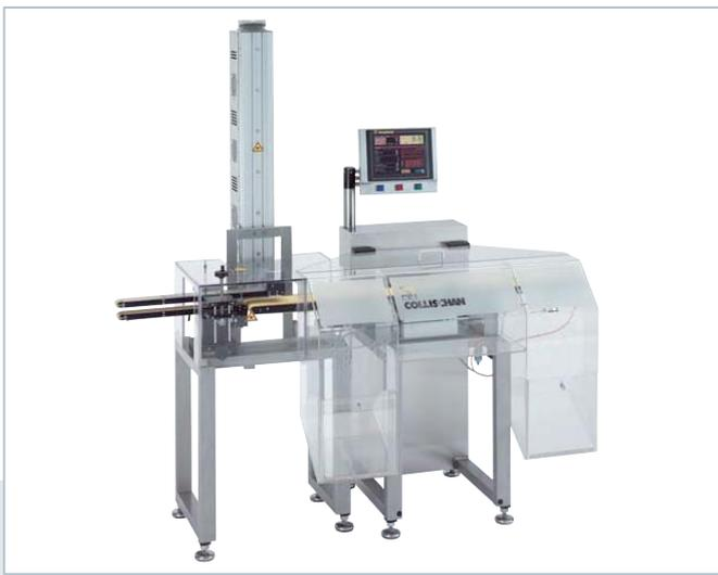
The **TC 8410** is a high speed checkweigher with many special features for the pharmaceutical industry. On the picture you can see the version with open flap detection, laser coding system and 21 CFR part 11 compliance.
