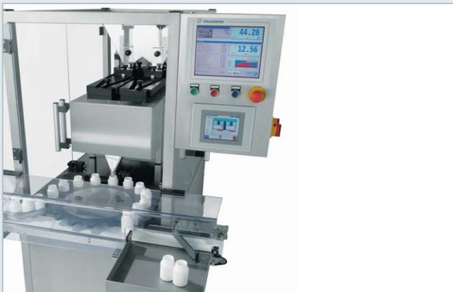
With the **TC 8210 Tare-Gross** each container is weighed before and after filling. The actual content is measured with high accuracy and weight deviations of the containers are eliminated. In conjunction with a counting machine, the combination of two different systems (counting and weighing) provides the maximum certainty to exclude an error.
