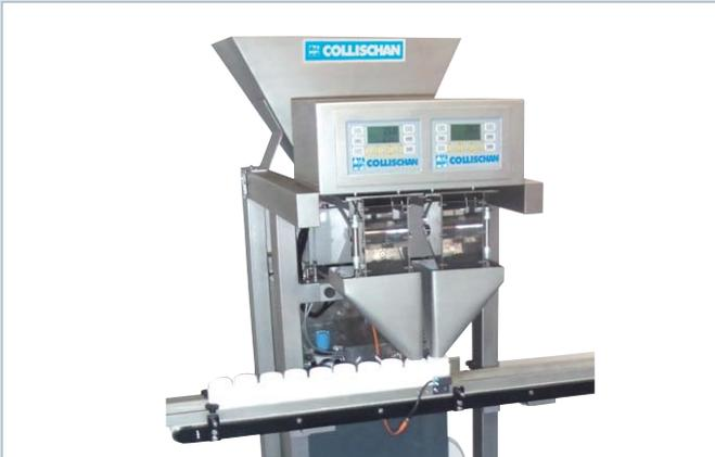
Twin Weigh filler **S 706-2** with automatic filling station for higher output. On demand the machine can be equipped with many weighing heads.
