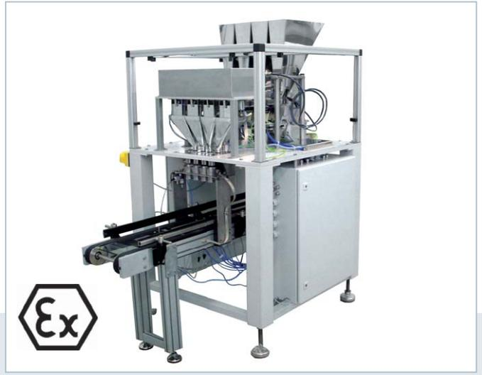
**Ex 706-4:** The multiple linear weigh filler doses explosives of 30.000 mg with an accuracy of  $\pm 3$  mg at a speed of approx. 25 weighings per minute.
