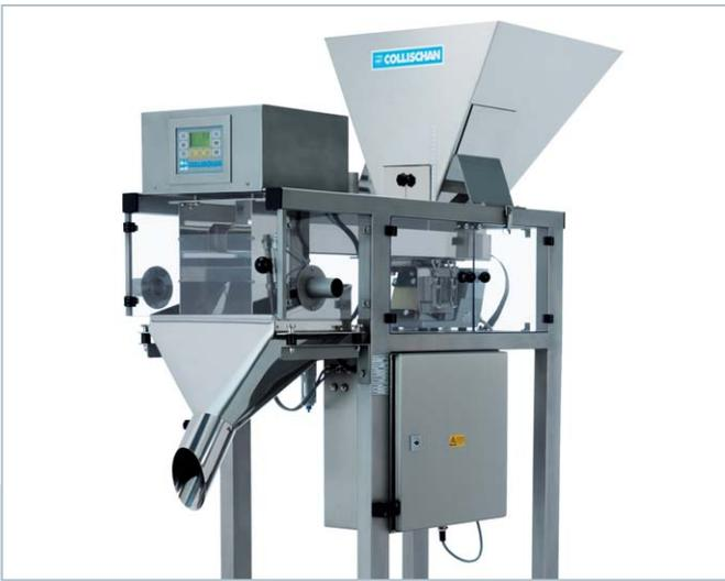
**S 710** for manual filling. Depending on the flow behavior and characteristics of your product, we provide different designs with weighing ranges from 50 g to 5000 g.
